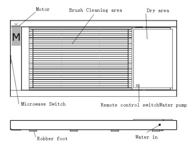
The sole cleaning machine adopts variable pole starting winding technology, convenient use, maintenance is simple, safe and effective. Staff through the cleaner can remove dirt, the soles of the bacteria completely off, and there is no need to change shoes and shoe covers.
